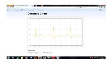
Fig. 6 ECG signal plotted in the browser of the laptop configured as server.
