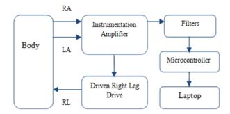
Fig. 2. Block diagram of ECG acquisition system
