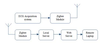
Fig.1. Block diagram of the system
