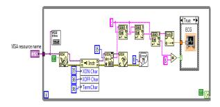
Fig. 3 Block diagram for ECG display in LabVIEW.
